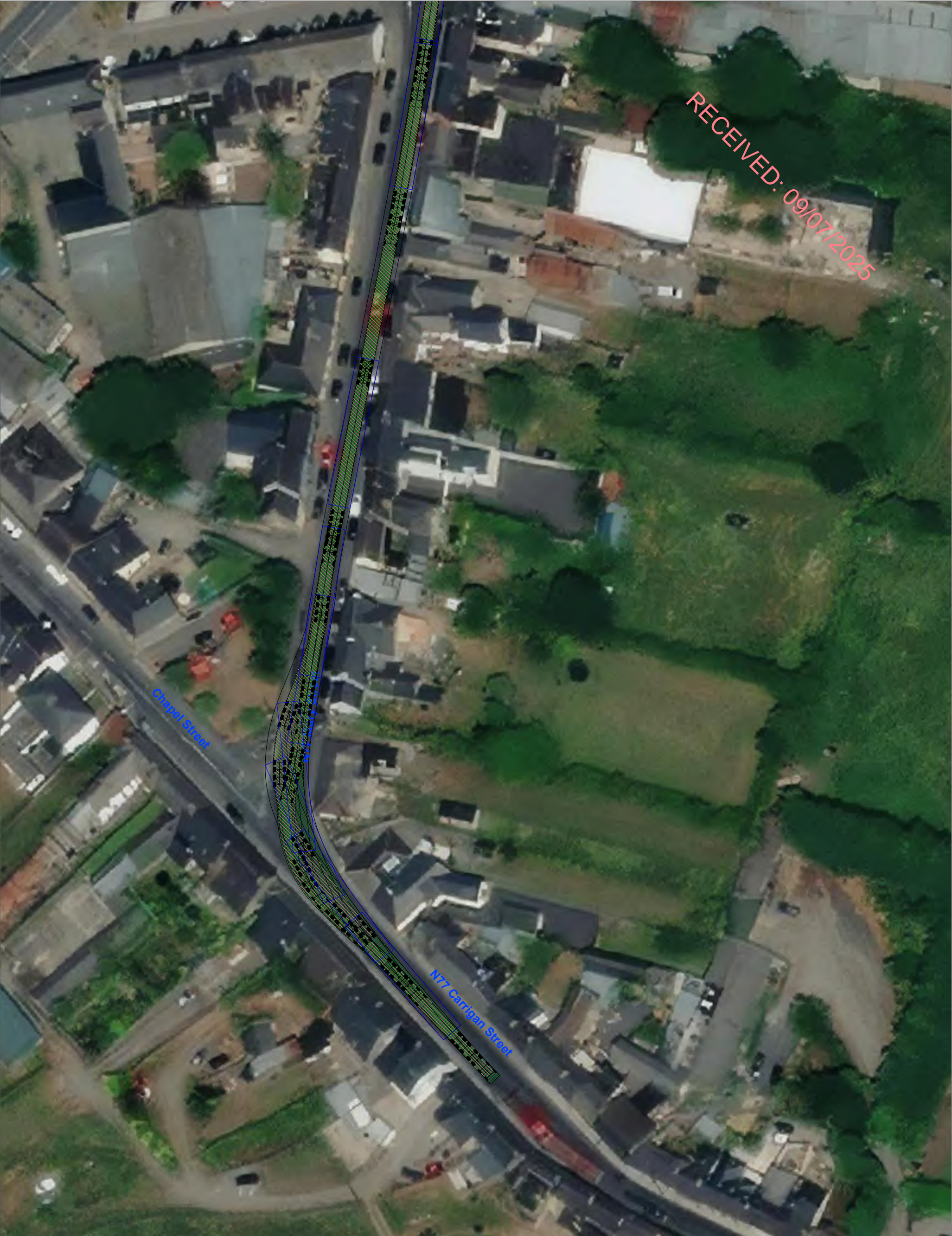
Figure 15-8 Location 1 - N77 Mary Street / N77 Carrigan Street / Chapel Street junction, autotrack assessment, tower extended artic
